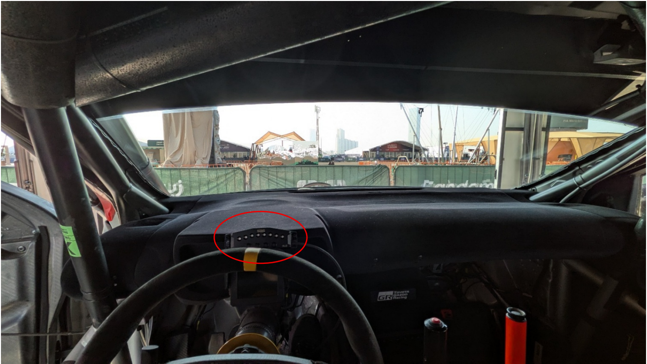
Figure 5. RLD device mounted just to the side of the vehicle's steering wheel
