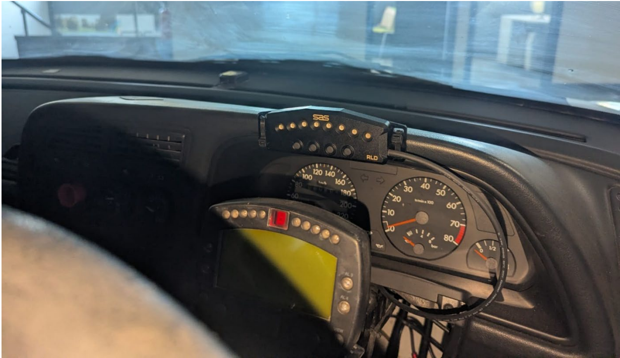
Figure 6. RLD device mounted directly in front of the driver
